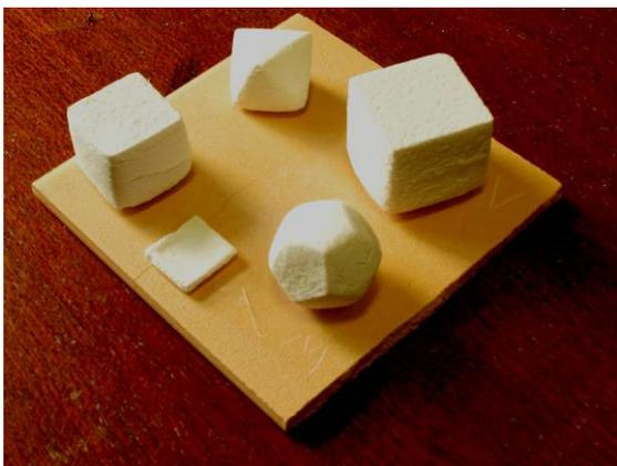
Figure 1 – Sintered 3D models printed in a 3D printer using a mixed powder containing glass frit, dextrene and sugar.
